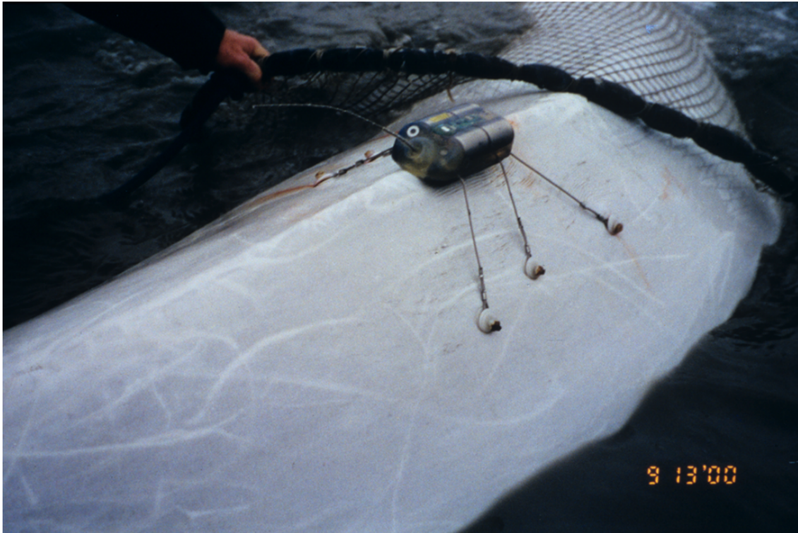
Figure 11. -- Whale CI-DL-03-00 (aka “Ringo”, alternate ID: CI-0001) outfitted with a satellite-linked time/depth recording (SL-TDR) tag attached via three nylon rods inserted through the blubber layer of the dorsal ridge.
