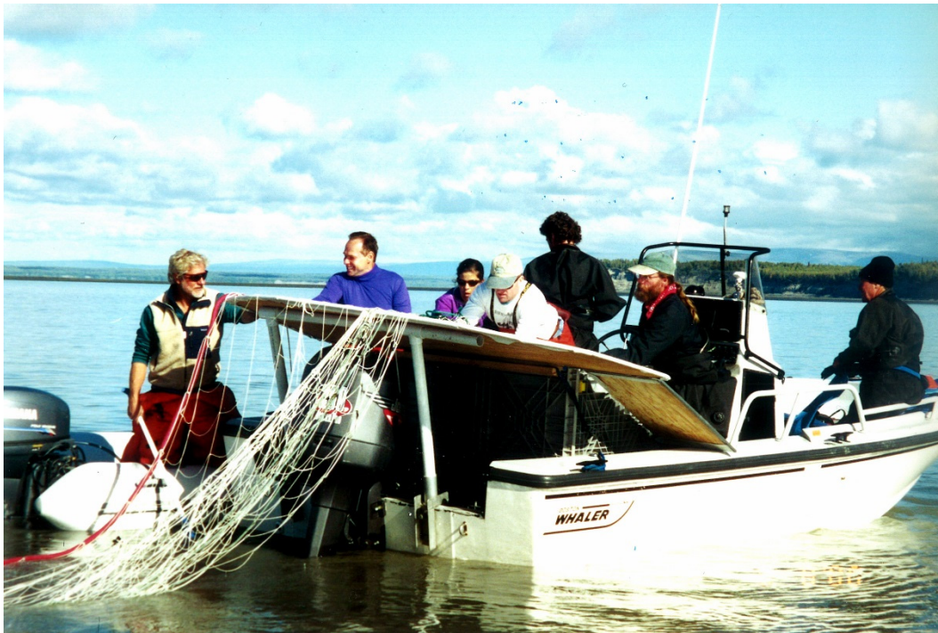
Figure 4. -- Ramp system used to deploy the capture net during the 2000-2002 Cook Inlet beluga tagging project.
